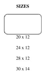
ALL pools have 2' Radius Corners REMEMBER! to allow for a 24" Overdig on each side of pool structure.
