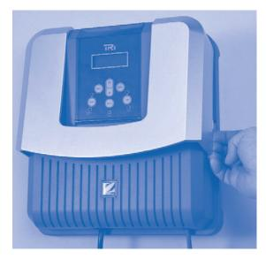
Remove the two screws that fix the lower module to the main unit (see below):
