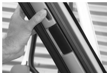
C3: To open, pull handles apart in the direction of the arrows and return to rest position in the A-pillars.
