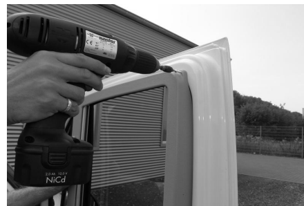
B30: Screw on side system using 6 self-tapping screws LIK 3.5x19 (Torx T10)
