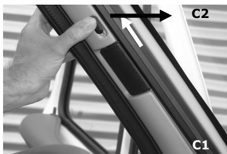
C1: Push button up in order to unlock front blind.
