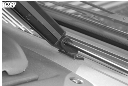
B27: Close blind to find position for lower tube carrier. Fix holder in this position using adhesive tape.
