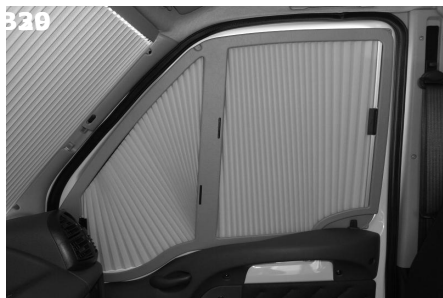
B29: Place the side system in the door frame and press on.
