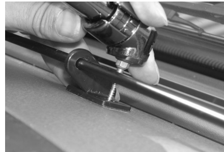
B28: Screw tube carrier onto the instrument panel with 2 screws SK 4.2x13.
