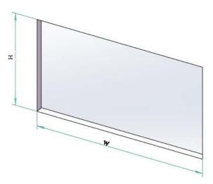
2.2 Step 2: And check whether the installation hole is standard. And please apply polyurethane sealant evenly to the border of the frame.
