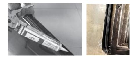
2.3 Step 3: Push the window into the installation hole from outside. Remove the protective film on the frame and press the window tightly. Align the mounting frame with the window from inside of vehicle and tighten them by screws while the personnel on the outside press the window.
