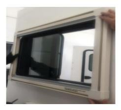
Step 7: Remove the PVC strip before installation.
