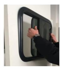
Step 4: To install the window to the vehicle, cross groove pan head self-tapping screws via the installation frame from the inside. Tighten screws crosswise.
