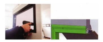
**04** Use self-tapping screws to install the window to the vehicle.
