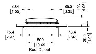
NOTE: Dimensions in millimeters [inches are in brackets]
