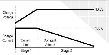
During stage 1 the battery voltage is increased gradually while the current is limited to start the charging process and protect the battery. At stage 2 the voltage rises to 13.8V to deliver the bulk charge to the battery. When the battery is charged, the float charge is maintained at 13.8V. The charger can be left switched on continuously as required.
