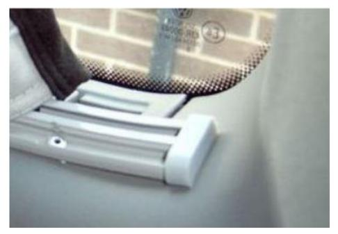
9. Now that the curtains are fitted, look at the end of the curtain with the poppers facing the outer edge as these need to be attached to the side of the window frame. To fit the 6 male poppers please fix where necessary with a rivet or the last remaining 6 screws included in this kit. (Please view the image below for an example how the male poppers on the window frame align with the female poppers off the curtains.)
