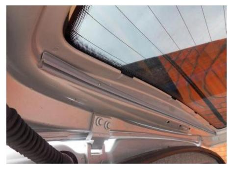
3. The L-Shaped rail fits along the bottom panel below the window for the tailgate door. (Refer to the image below.) Please note: Leave some clearance for your bottom rail if the vehicle has a wiper motor fitted.
