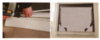
Install the blinds to the vehicle with cross groove countersunk head self-tapping screw provided via the installation groove.
