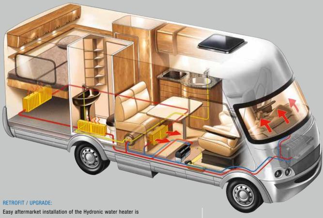
Easy aftermarket installation of the Hydronic water heater is possible in the engine compartment. The heat is evenly distributed through the vehicle's own air ducts, additional radiators or blowers.
