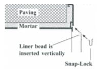
The U.K or U.S.A manufactured liner will clip into the receptor and hang vertical and not horizontally as conventional liner locks do. Aluminium coping also eradicates the unsightly undulations that can appear between conventional liner lock and underside of stone copings.
