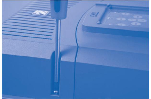
Gently remove the lower module from the TRi unit.
