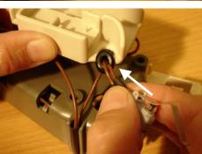
Pull back the cable into the saddle.
