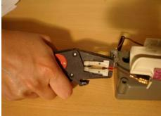
Strip the both wires with a wire stripper.
