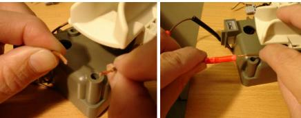
Connect the connectors from the new switch on the cables with the shrink pliers.
