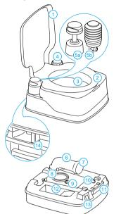
1 Cover • 2 Seat • 3 Toilet bowl • 4 Water filler cap • 5a Piston pump • 5b Bellow pump • 6 Pour out spout • 7 Cap pour out spout • 8 Lip seal • 9 Vent seal • 10 Vent button • 11 Valve handle • 12 Storage for toilet fluids • 13 Level indicator waste-holding tank (dependent on model) • 14 Clasp
